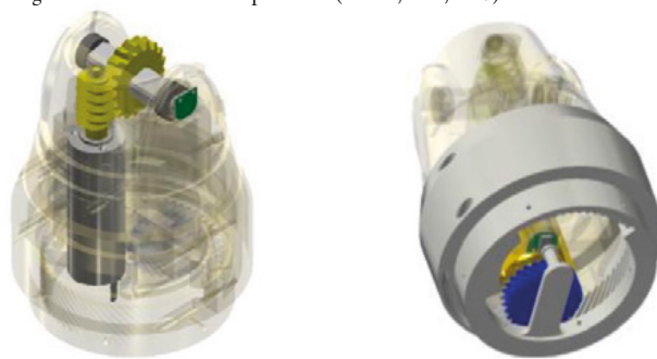
Figure 14. Detail of the wrist design of the Octa Hand prosthesis (Abarca, et al., 2019).
