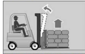
4. Raise the carriage about one inch. Slowly tilt the mast to a vertical position as you scoop up the load.
