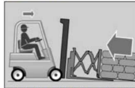
3. Move forward slowly as the load is being pulled onto the platen.
