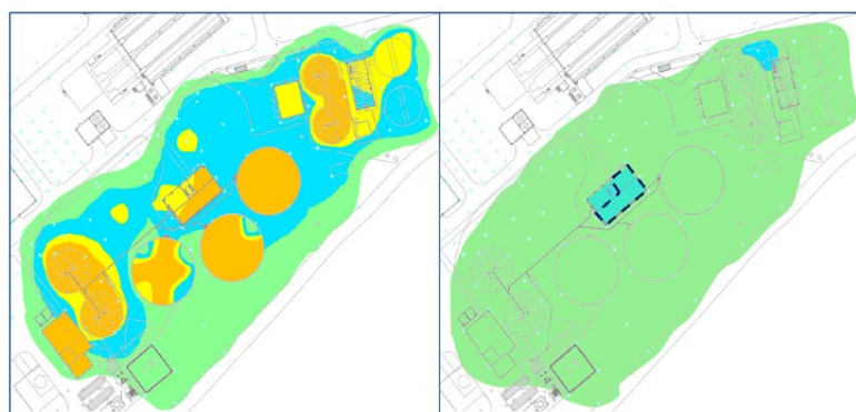
Figure 5. Concentrations of H 2 S (left) y relative humidity (right) in sludge line.
